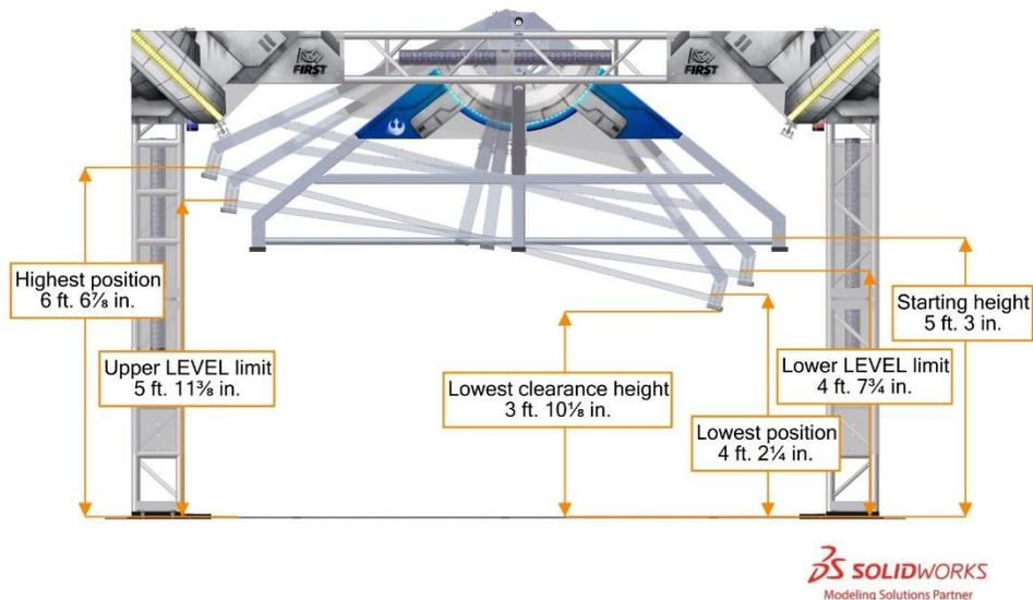
Figure 3-9 GENERATOR SWITCH range of motion
