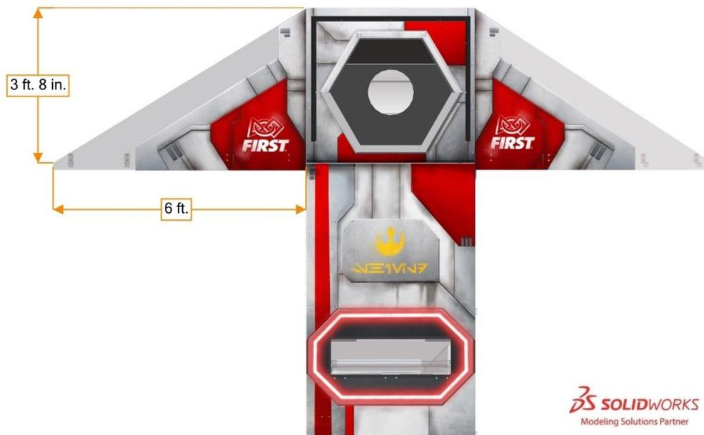
Figure 3-16 Backboard dimensions
