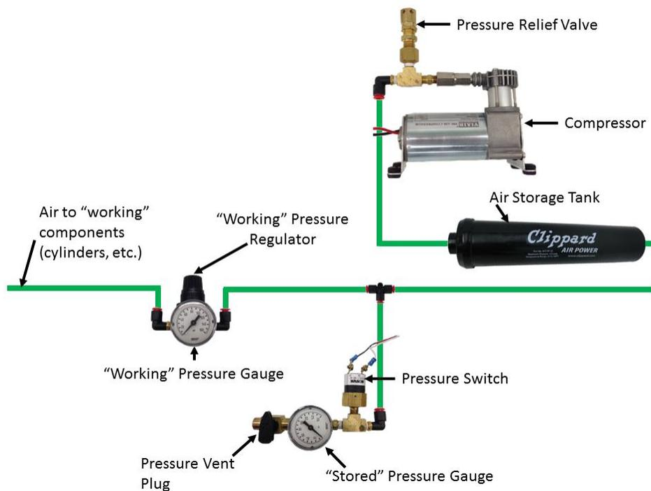
Figure 9-15 Pneumatic circuitry
